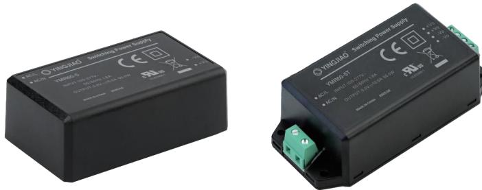
YMR60 is a 60W miniature (87\*52\*30mm) AC-DC module-type power supply, ready to be soldered onto the PCB boards of various kinds of electronic instruments or industrial automation equipments. This product allows the universal input voltage range of 85~305VAC.
