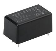
YMR5 is a 5W miniature (46.08\*25.78\*21.7mm) AC-DC module-type power supply, ready to be soldered onto the PCB boards of various kinds of electronic instruments or industrial automation equipments. This product allows the universal input voltage range of 85~305VAC.
