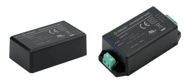
YMR45 is a 45W miniature (87\*52\*30mm) AC-DC module-type power supply, ready to be soldered onto the PCB boards of various kinds of electronic instruments or industrial automation equipments. This product allows the universal input voltage range of 85~305VAC.
